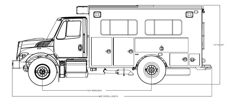
International MV607 330Hp Cummins H0 Bostrom crew seating 10 person seating 60,000 BTU/HR Crew heating and cooling Whelen Emergency lighting FRC True Sight 130 degree backup camera
